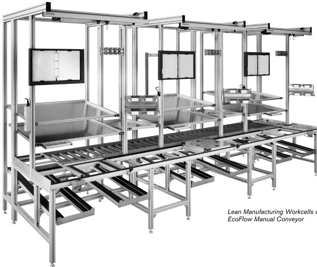
*Lean Manufacturing Workcells with EcoFlow Manual Conveyor*
