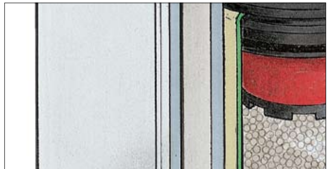
Corrosion protected by alocrom and epoxy painting.
