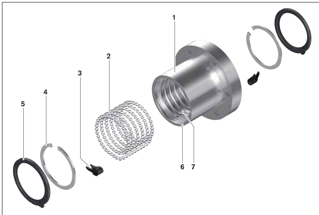
Structural design of a ball nut
