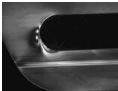
Fig. 5a Back Lit Plastic Film w/Crossed Polarizers
