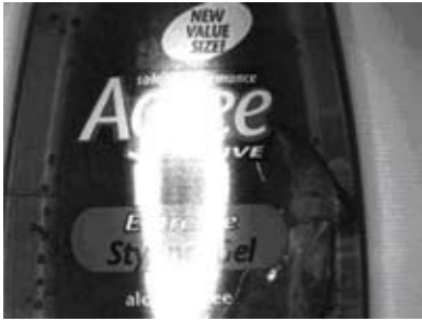
Fig. 3b Coaxial Ring Light - No Polarizer
