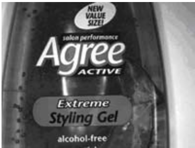
Fig. 3c Coaxial Ring Light w/Crossed Polarizer
