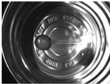
Fig. 2a - Off Axis Spot Light
