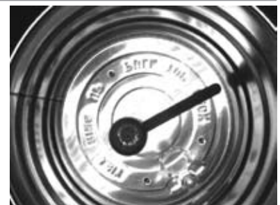
Fig. 2b - Co-Axial Ring Light
